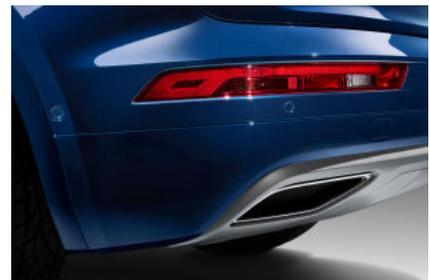
Rear retrofit solution for the parking system measures reversing distance with four ultrasonic sensors.
