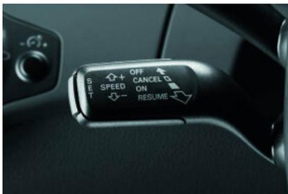
Retrofit solution for the cruise control system maintains any speed as of approximately 30 km/h.
